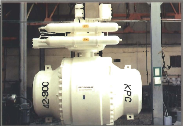
KPC 3 PIECE TRUNNION VALVE FOR OFF SHORE SERVICE. (42" 900 ANSI - 60,000 LBS)
